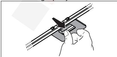
**Type 15 - NON-washable activated charcoal filter** - The saturation of the charcoal filter occurs after more or less prolonged use, depending on the type of cooking and the regularity of cleaning of the grease filter. In any case it is necessary to replace the
