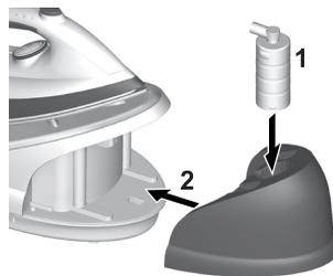
**6. Insert the water tank** into the base unit. Ensure that the water tank latches securely into place.
