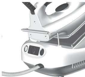
**2. When the power switch is pressed,** the power lamp will light. Wait for one to two minutes, until the steam lamp lights.
